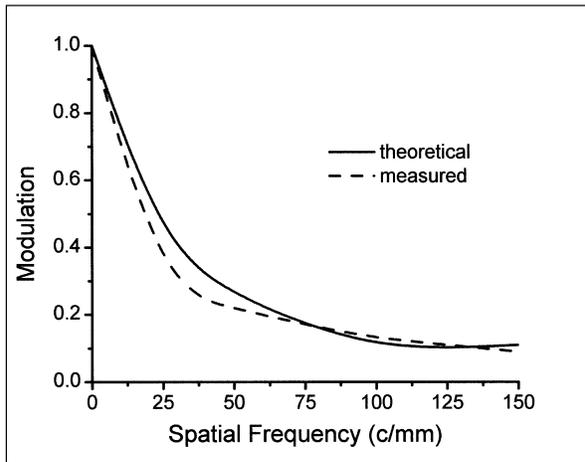
**Figure 2.** The theoretical and measured through-frequency modulation transfer function (MTF) of the physical cornea model (for a 5-mm pupil diameter).
