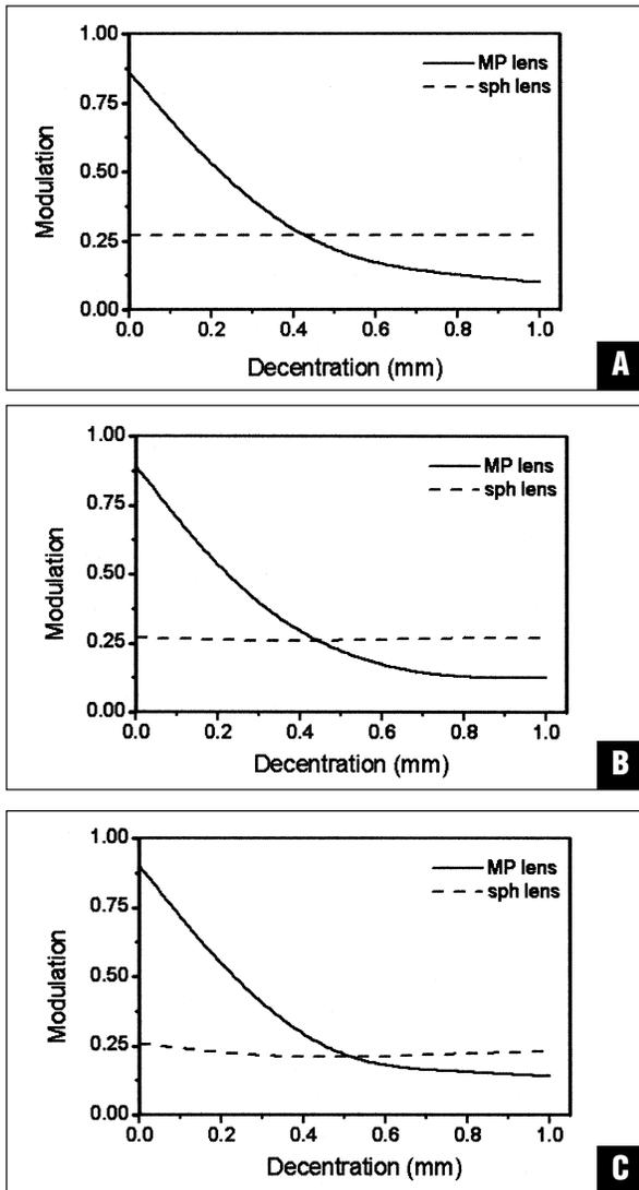
**Figure 7.** The ocular MTF as a function of lens decentration for the modified prolate and spherical lenses. MTF was calculated in the model eye at 50 c/mm for a 5-mm pupil diameter (average values for the meridional and sagittal directions). **A)** 5-D lenses; **B)** 20-D lenses; **C)** 30-D lenses.
