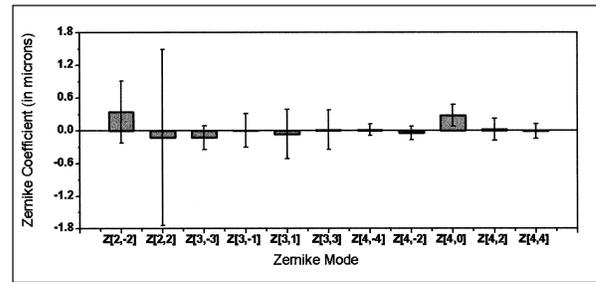
**Figure 3.** Average values of Zernike aberration coefficients for the cornea for a 6-mm aperture diameter (in microns). The error bars are representative of  $\pm 1$  standard deviation.
