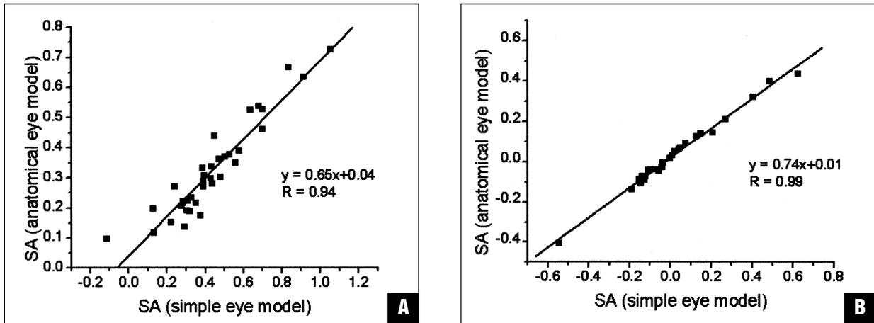
**Figure 5.** The correlation between the spherical aberration calculated using the simple eye model and the spherical aberration calculated using the eye model constructed with anatomical data. **A)** Pseudophakic eye models containing spherical IOLs; **B)** Pseudophakic eye model containing the modified prolate IOLs.
